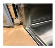
A stainless steel threshold ramp(s) is included to facilitate rolling in racks. It is shipped wrapped in brown paper and secured to the rack guides inside the cabinet. To secure in place, remove the two thumb screws in the breaker strip near the bottom door opening. Place the ramp(s) on top of the loosened thumb screws and secure tabs on each end to the breaker strips with the thumb screws previously removed. After installing the ramp(s), it too should be sealed to the floor.
