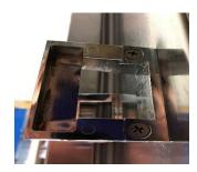
To adjust the lockkeeper you will need to remove the two screws holding the lockkeeper. Loosen the two screws in the bracket mounted on the cabinet but do not remove them. The bracket can be move slightly from side to side. Tighten the screws in the bracket and replace the lockkeeper. Make sure the lock bolt catches the lockkeeper so the door can be locked.
